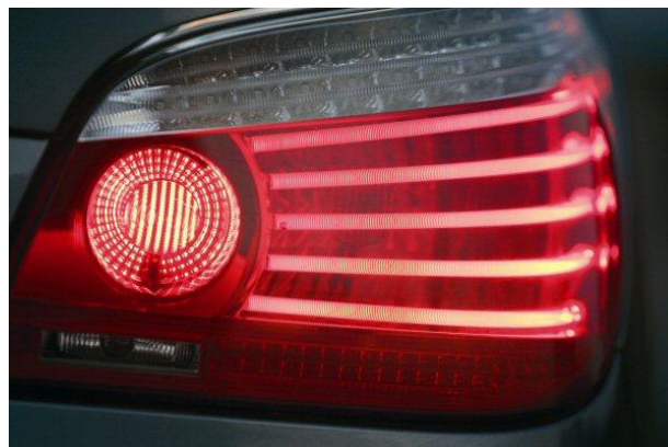
Textured light guides of a tail lamp
